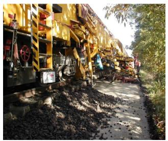
Encase of cleaned railroad balast after cleaning path
