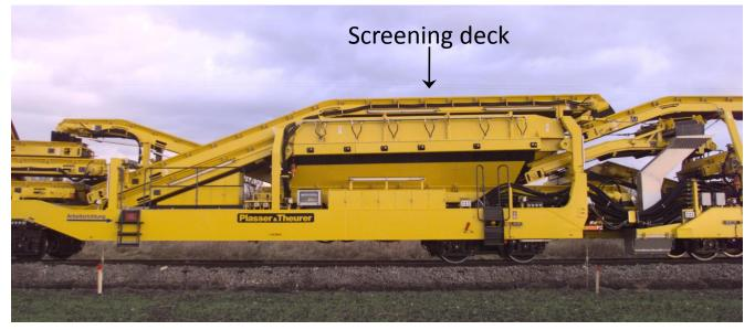
Remove of contaminated railroad balast from railway
