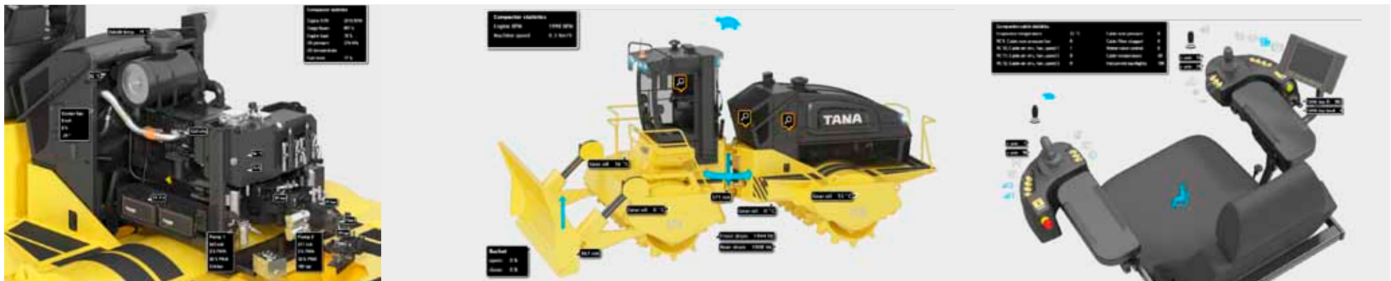
TANA SMART SITE™ offers a tool for viewing the status of the compactor and details of the power pack components over the internet in real time.
