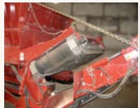
NEOFLUX® overbelt magnet on wood shredder (lightweight and compact)
