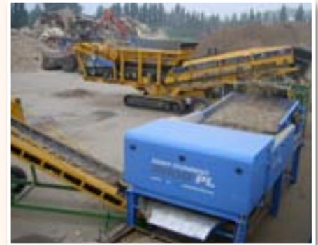
*Non-ferrous separator with a width of 2000 mm for processing of waste wood*
