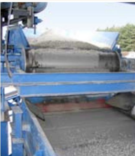
NEOFLUX® drum magnet for glass recycling
