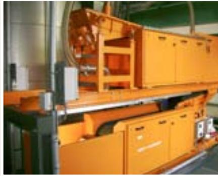
Non-ferrous separator in the shape of a cascade for the separation of 2-10 mm metal particles from slag
