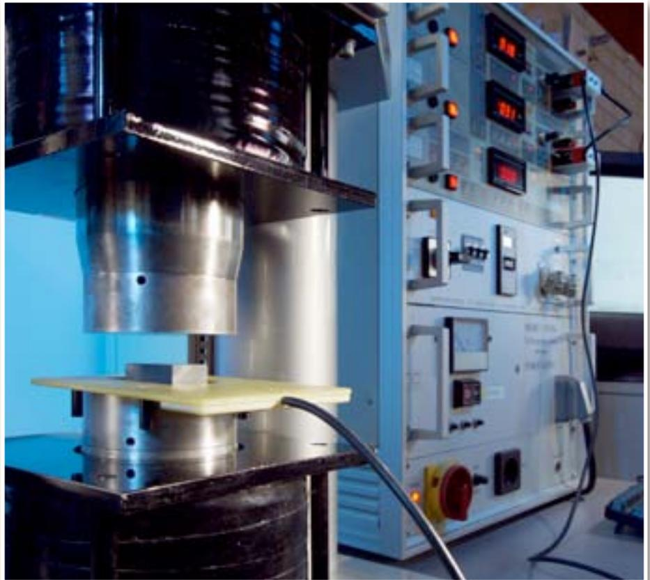
*A Permagraph determines the magnetic energy*
