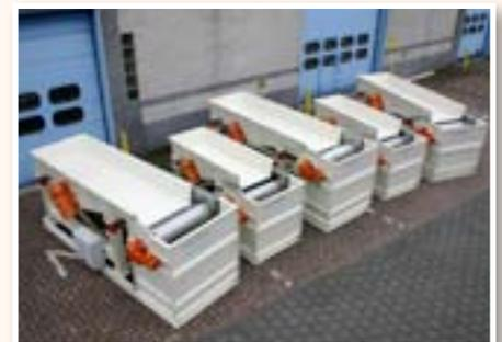
NEOFLUX® drum magnets with vibrating chute
