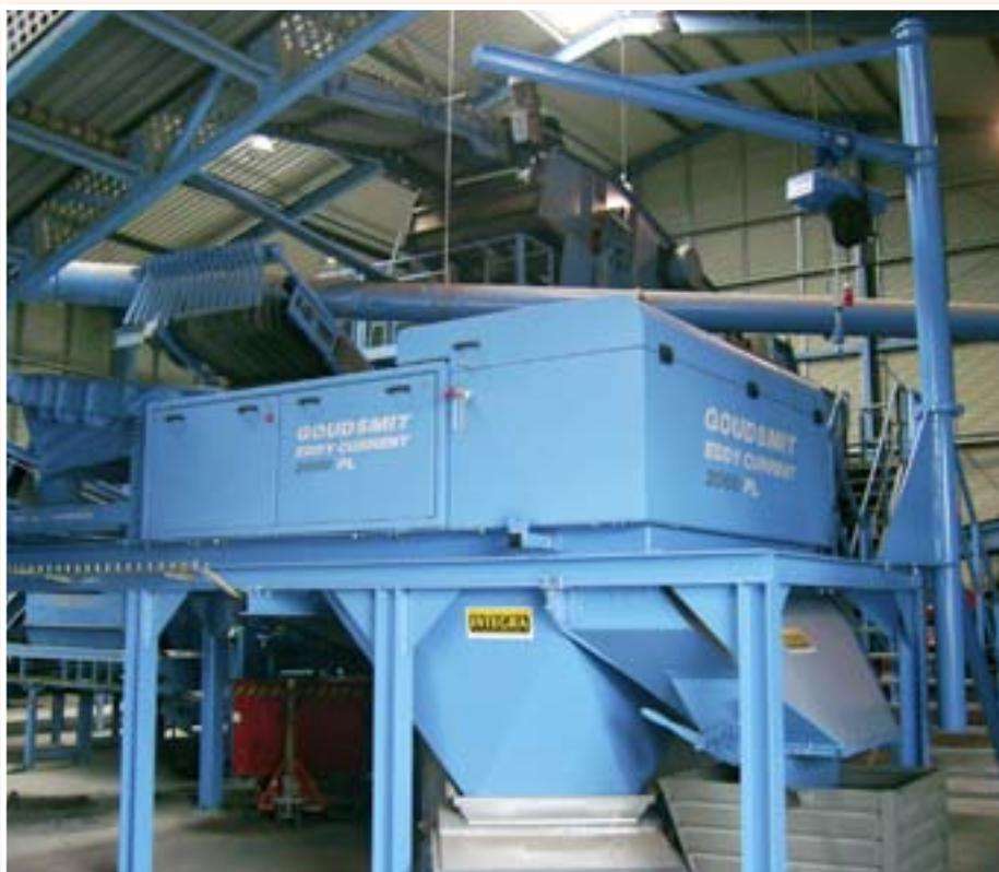
*Non-ferrous separator type NF2000 in combustion slag fraction*
