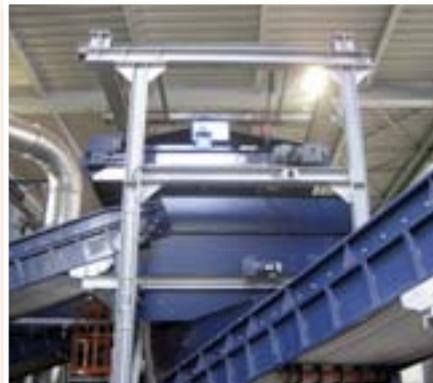
Electro overbelt magnet for construction and demolition waste
