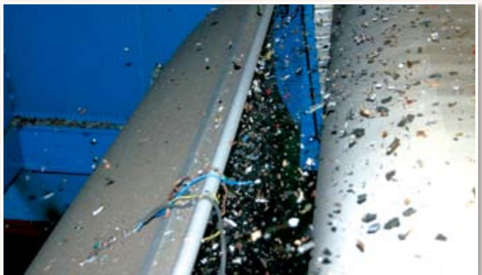
Detail of non-ferrous separator (width: 1500 mm) for WEEE scrap
