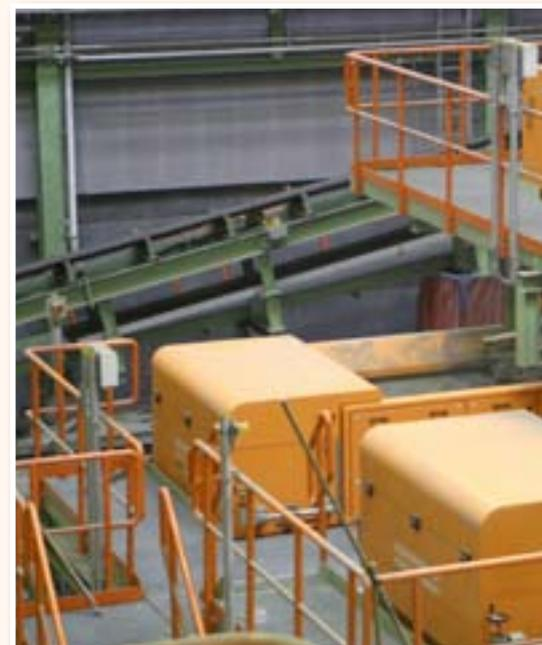
*Three non-ferrous separators type NF1500 on plateau in combustion slag reprocessing*
