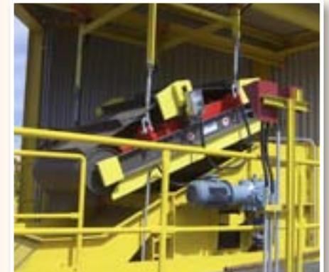
Electro overbelt magnet for the wood processing industry
