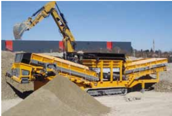
Starscreen with 2 long screen decks in soil with clay portion
