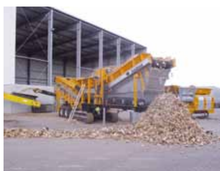
Screening of old wood after upstream coarse crusher
