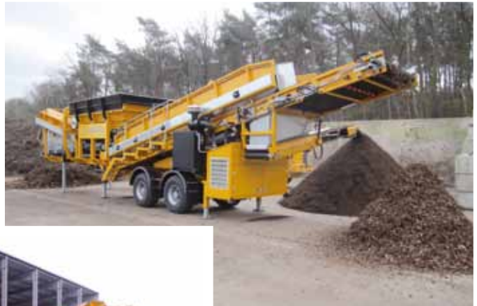
Screening of old wood after upstream coarse crusher
