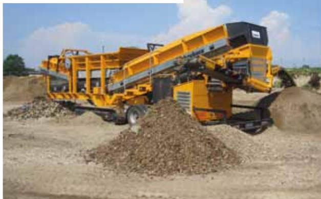
Starscreen and mixing machine as screen machine in soil with rock portions
