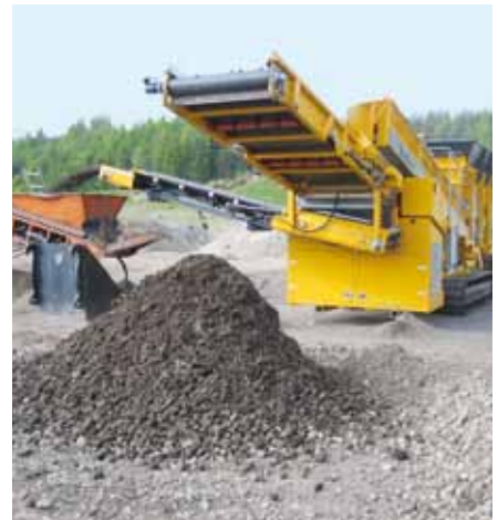
Soil screening with hauling away the fine grain by external conveyor
