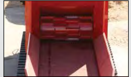
Gap-less infeed transition
